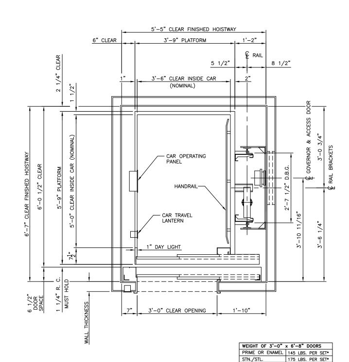
\*INCLUDES WEIGHT OF (1) SET OF DOORS ON CAR OR HOISTWAY (TOTAL WT. OF DOORS WITH STN/STL CAR DOORS AND PRIME ENTRANCE DOORS IS 320 LBS.)
